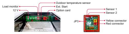
Fig. 20. Couplings on the boiler circuit board
